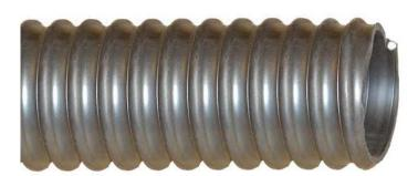
The Model PH1 is a high quality, heavy duty SBR rubber blended with static carbon black and rigid PVC helix material handling hose. It provides quiet operation, excellent bendability, and good abrasion resistance that has a smooth bore. It is made for transferring and suction of dry materials, and dissipates static.
